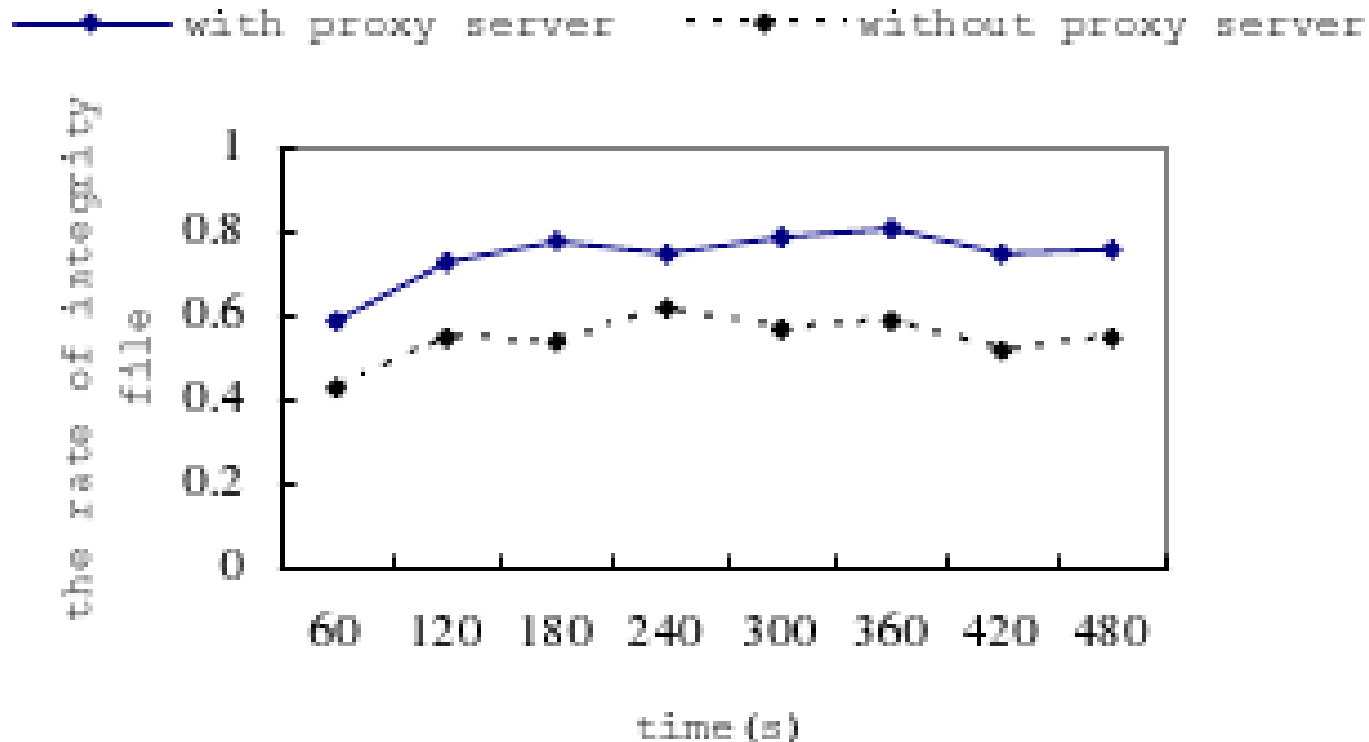
Figure: The file integrity rate under the situation of with proxy server and without proxy server
